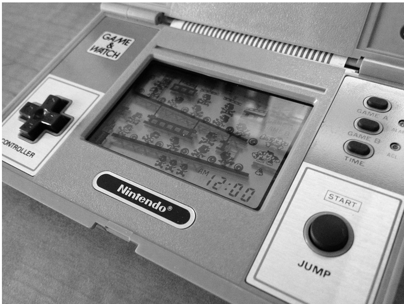
1.2 The lower screen of the Game & Watch Multi Screen Donkey Kong handheld, the first Nintendo product to feature the "Plus" Button. In its startup state (pictured), one can see the entire spectrum of LCD segments lit simultaneously.
